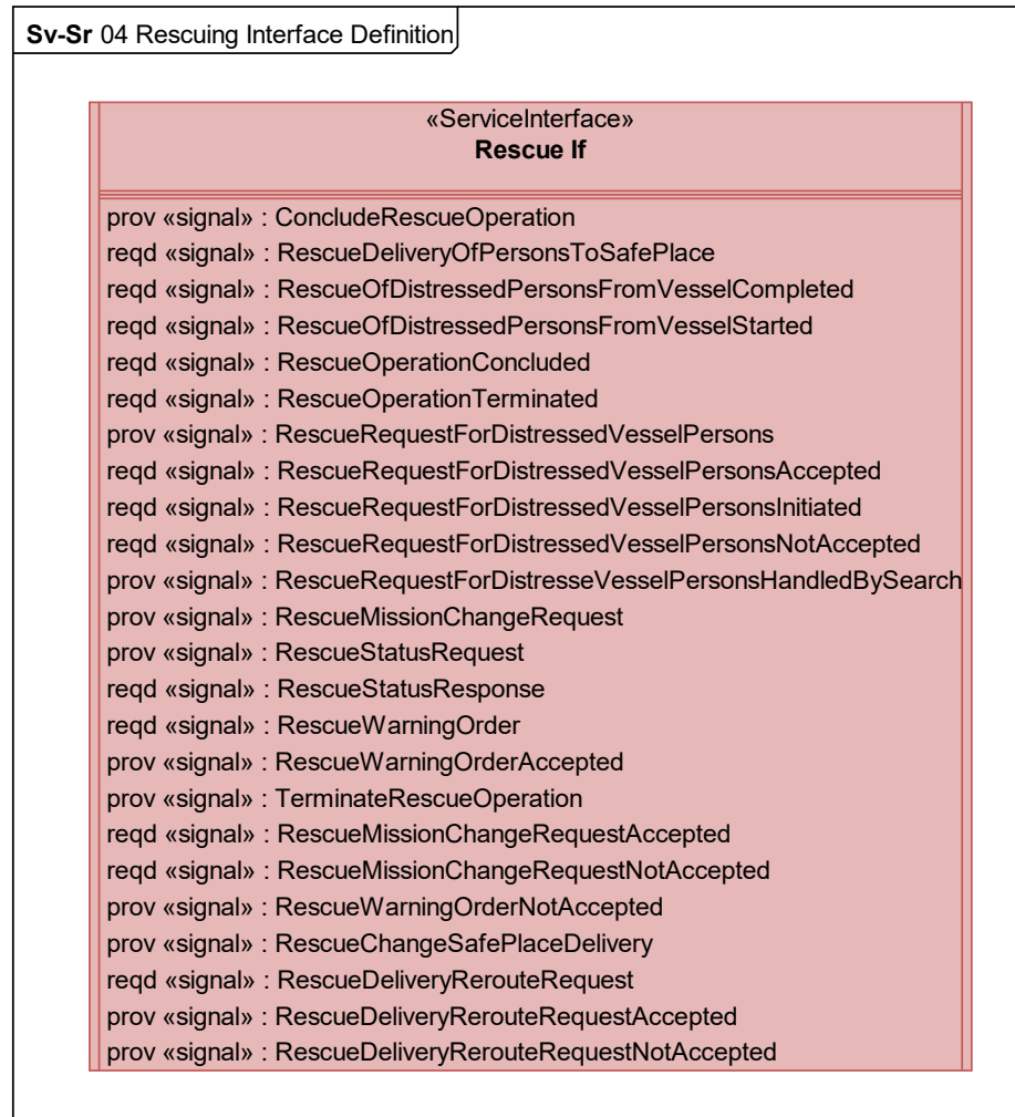
Figure 17:6 - Services Structure for the Rescue Interface
